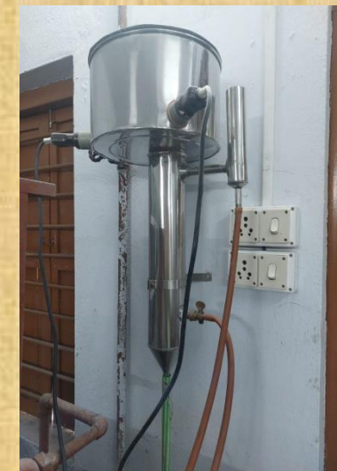
Hanging Water Distillation Plant
